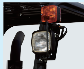
LED Head lamps (with guard)
