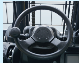
Small diameter steering wheel (11.8")
