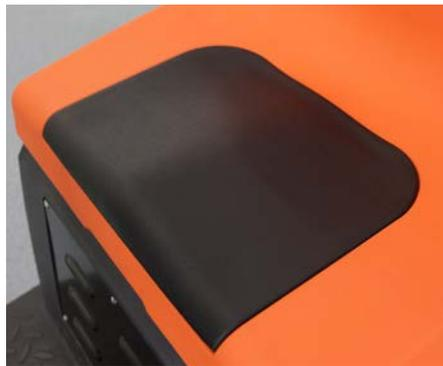
Operator Presence System (OPS) — When operator is not in seat, the scrubber will automatically stop.
