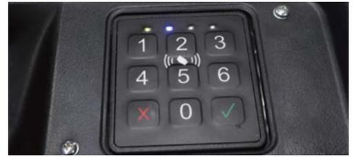
Keyless PIN code lock or RFID card access simplifies access when several users operate one truck.
