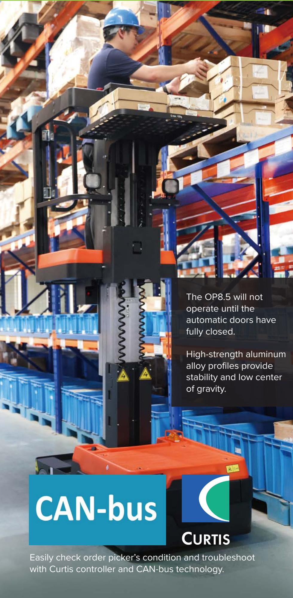
The OP8.5 will not operate until the automatic doors have fully closed.
