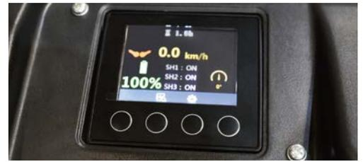
LCD display shows safety warnings, speed, steering angle and fault codes for easy operation and troubleshooting.
