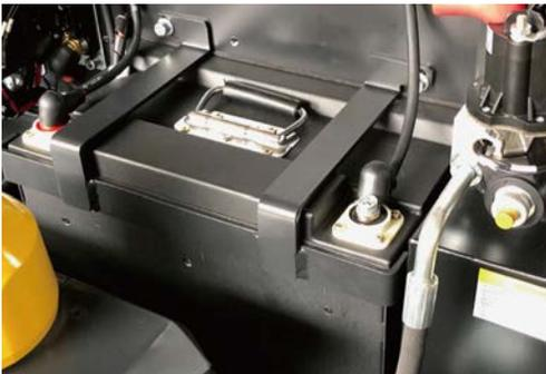
24V/80Ah Lithium-iron battery has connection terminals with screws and is protected inside the steel case.
