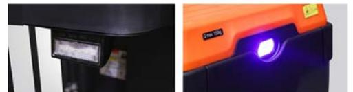
Side lights and headlight provide excellent visibility to operator even in poor lighting conditions. Vehicle is also equipped with a buzzer, warning light, rear light and safety blue light.
