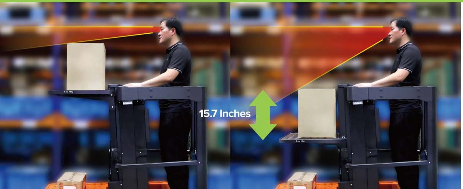
Adjustable front shelf can be raised and lowered to ensure operator's field of view is not obstructed.
