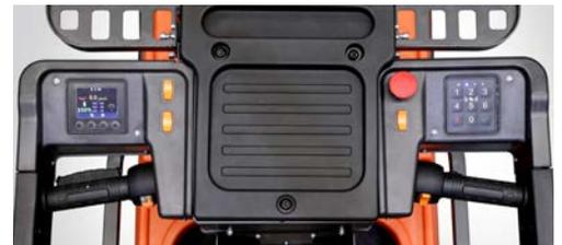
Left and right multi-function handles can be customized and provide simultaneous lifting, traveling and steering. Handles are equipped with operator presence buttons to ensure safe operation.
