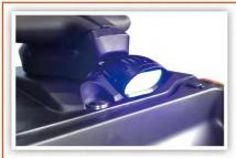
The standard blue light is mounted in a way that highlights the path the truck is taking. Greatly improving pedestrian safety.
