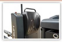
Safety flanks and non-slip materials on both sides of the backrest ensure operator safety during operations. Ergonomic handle to assist in entry and exit of operators compartment
