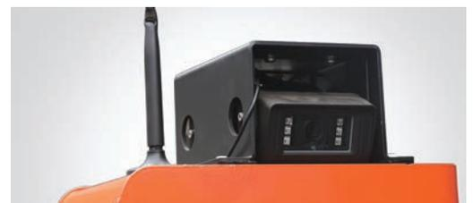
The dual-screen, 3-camera, high-definition monitoring system allows the operator to monitor cargo stacking in real time.
