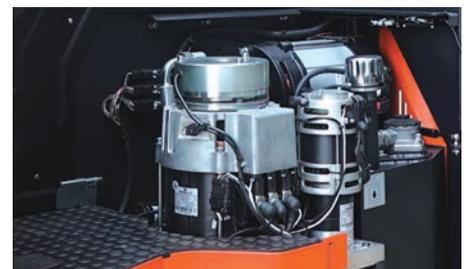
Low-noise gear pump ensures quite lifting. Motor controller, oil pump motor controller and steering motor controller, provide self-protection, maintenance-free, superior performance.
