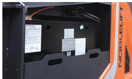
Large capacity battery provides multiple shift operation. Side extraction reduces maintenance time.
