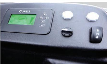
The multi-function, color LCD instrument panel can display the steering wheel position, battery power, power alarm, fault code, working time, driving speed and other information.
