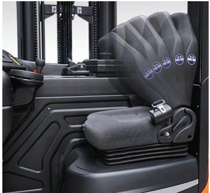
High suspension, fully adjustable seat reduces vibration to the driver. Together, with the automobile-type bionic curved backrest, they effectively reduce driver fatigue for all sizes of operators.
