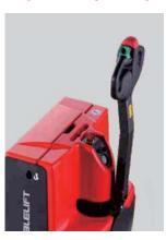
In particular through the long tiller design the operator can always keep a safe distance to the truck during proceeding the work very ergonomically.
