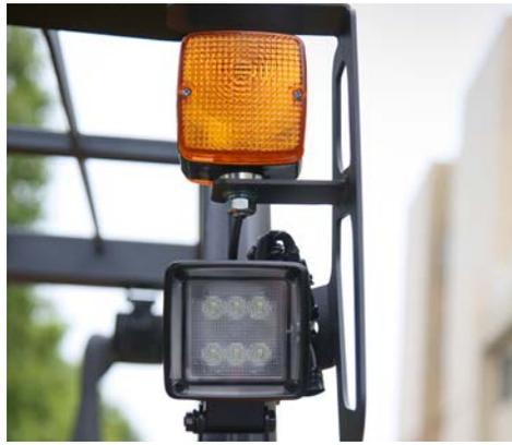
Equipped with LED lamps: LED rear work lights, headlights, strobe and safety blue light. Bright light with low power consumption provides excellent visibility.
