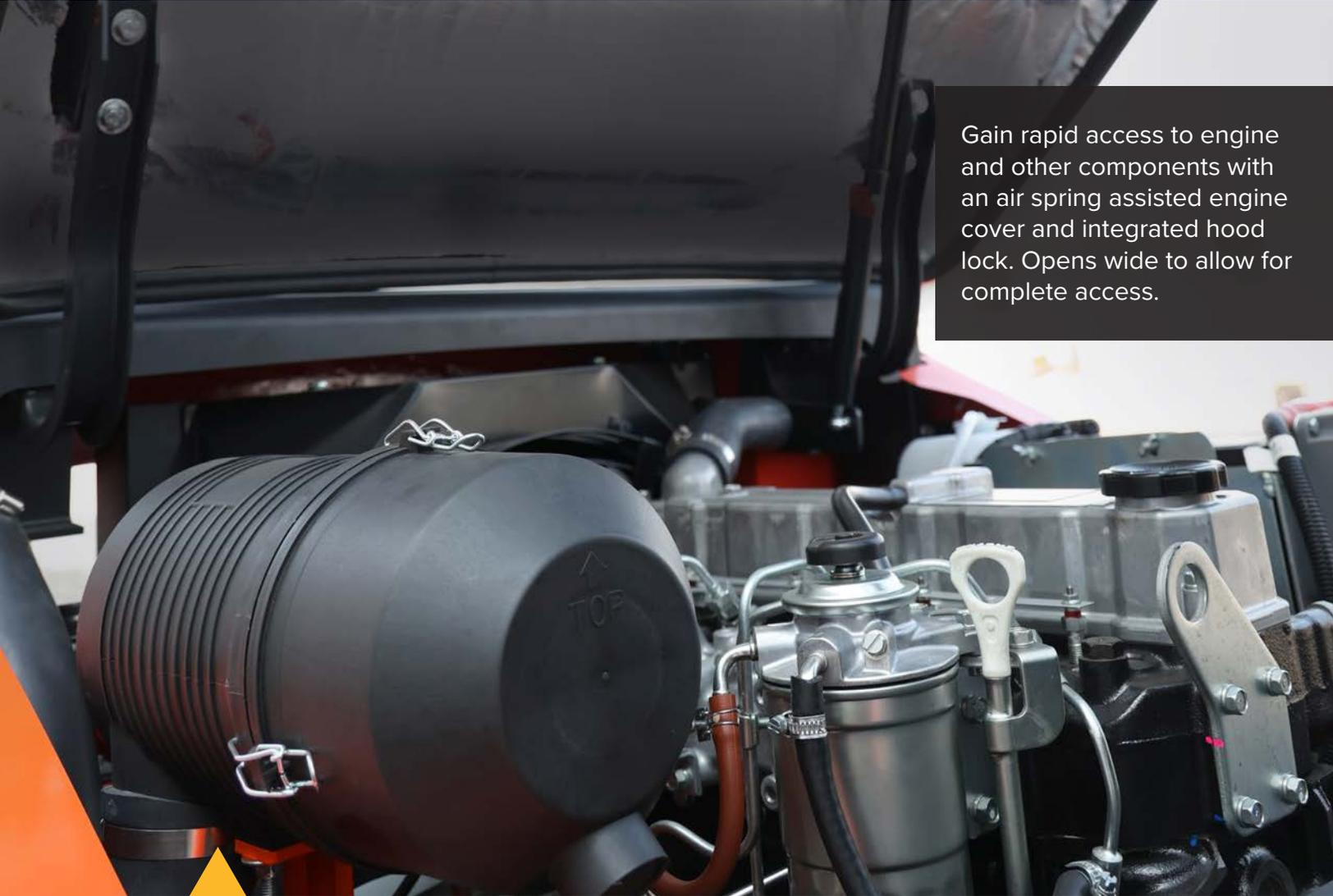
Gain rapid access to engine and other components with an air spring assisted engine cover and integrated hood lock. Opens wide to allow for complete access.
