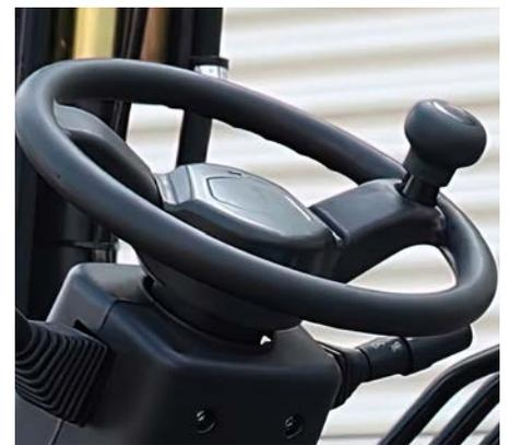
On-Demand Fully Hydrostatic Power Steering (FHPS) guarantees smooth steering, preventing over-run and kick-back. Spinner knob allows easier one-handed steering.
