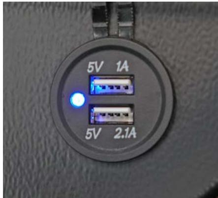
(2) USB connectors for charging and powering of additional devices during operations.
