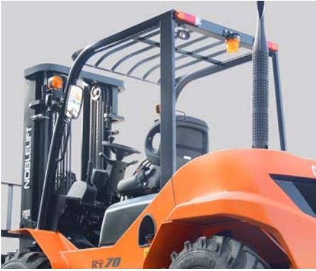
Heavy-duty steel chassis, axles, mast and overhead guard deliver high strength and stability for lifting heavy loads on the toughest terrain.
