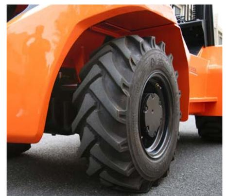
Large diameter, pneumatic tires ensure comfortable driving. Tire fender designed to prevent mud from getting in cab.
