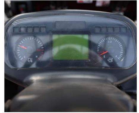
Large LED display and CAN Bus function provides truck status information: parking brake, driving direction, speed, hour meter and fault codes.
