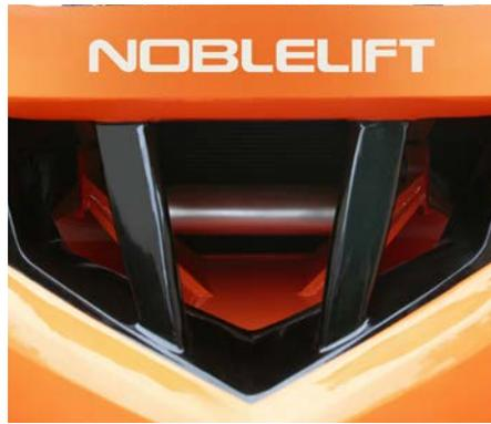
Optimized heat dissipation channel allows for larger radiator, keeping engine running reliably, even in the most demanding applications.
