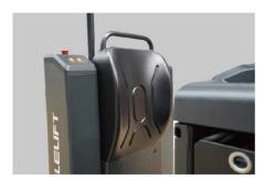
Safety flanks and non-slip surface materials on both sides of the backrest ensure the operator not to be thrown off while the truck turns at high speed. This design greatly improves the safety of driving.Meanwhile, the handle above the backrest provides a grasping point for the operator while getting on/off the truck, provides superior comfort for the operator.
