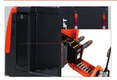
Sideways battery exchange compartment plus adjustable handling bracket makes battery replacement easier and guicker.
