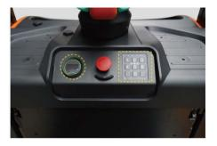
The multifuctional control instrument pin code switch can display truck conditions, battery capacity, working time, travel speed and steering angle. When something goes wrong, the outer ring light of the instrument will turn to red from green, and the fault code will be displayed.
