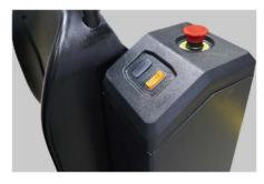
The coasting button on both sides of the truck and emergency stop button allow the operator to operate truck forward/backward while walking beside. There is no need to get in and out of the truck frequently to operate it.At the same time, it reduces the speed while driving forward/backwards under coasting mode, making the traction safer and more efficient.
